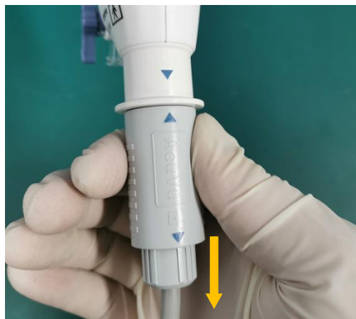
Figure 9 How to pull out the cable connector from the hysteroscope
