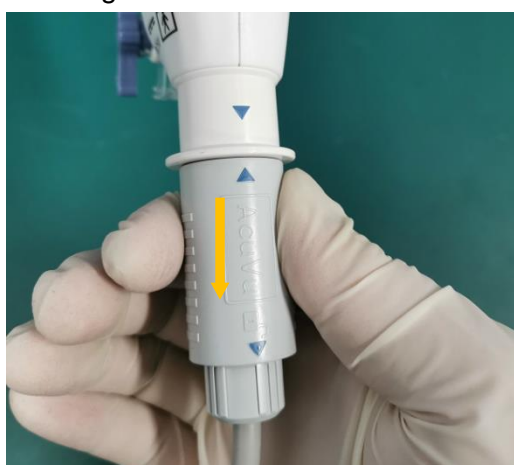
Figure 16 How to pull out the cable connector from the hysteroscope
